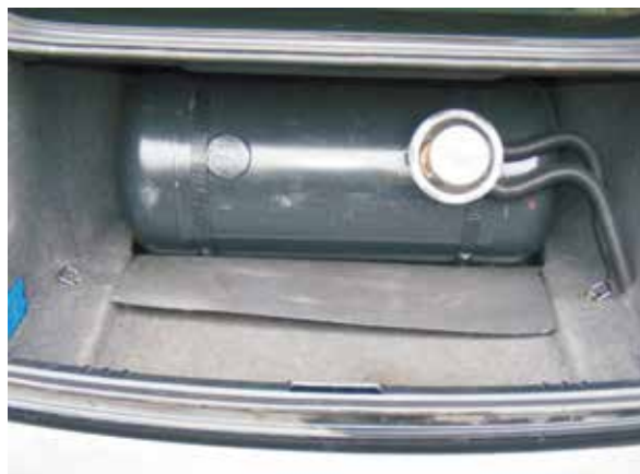
Fig. 10 Cylindrical tank behind the backseat
