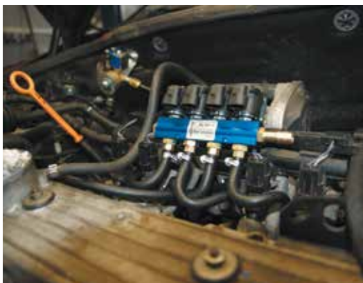
Fig. 3 Installation of injectors in the engine compartment
