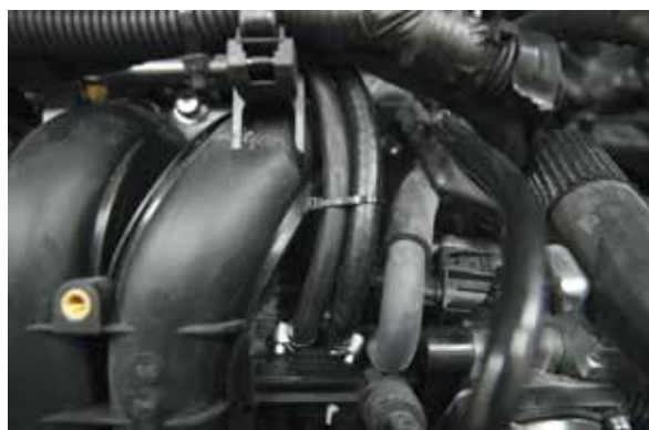
Fig. 13 Vacuum from the manifold downstream the throttle
