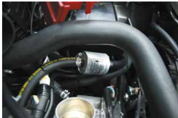
Fig. 12 Fixing the volatile phase filter
