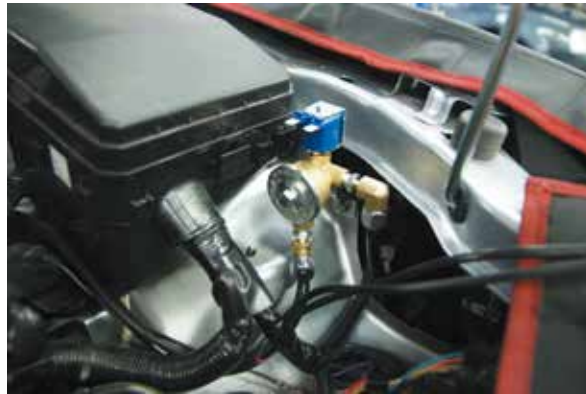
Fig. 7 Solenoid valve installation
