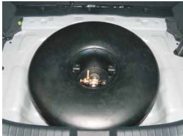
Fig. 9 Toroidal tank installed in the spare wheel compartment
